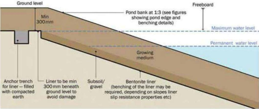
Figure 23.13 Details for a typical geosynthetic liner
