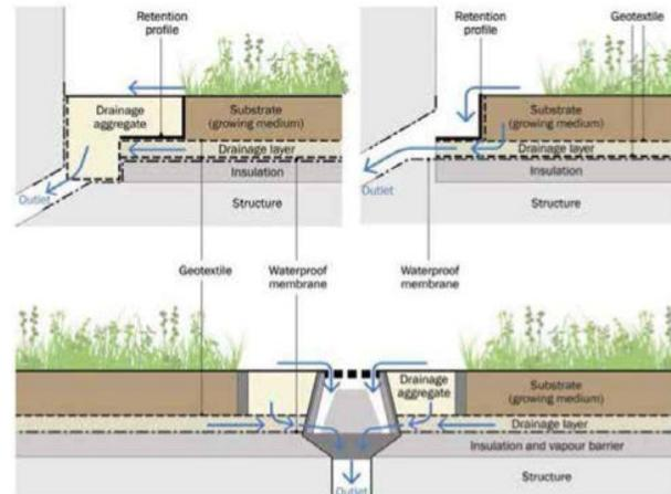
Drainage systems for an extensive green roof.
