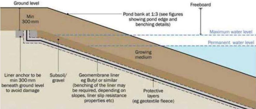
Figure 23.14 Details for a typical geomembrane liner
